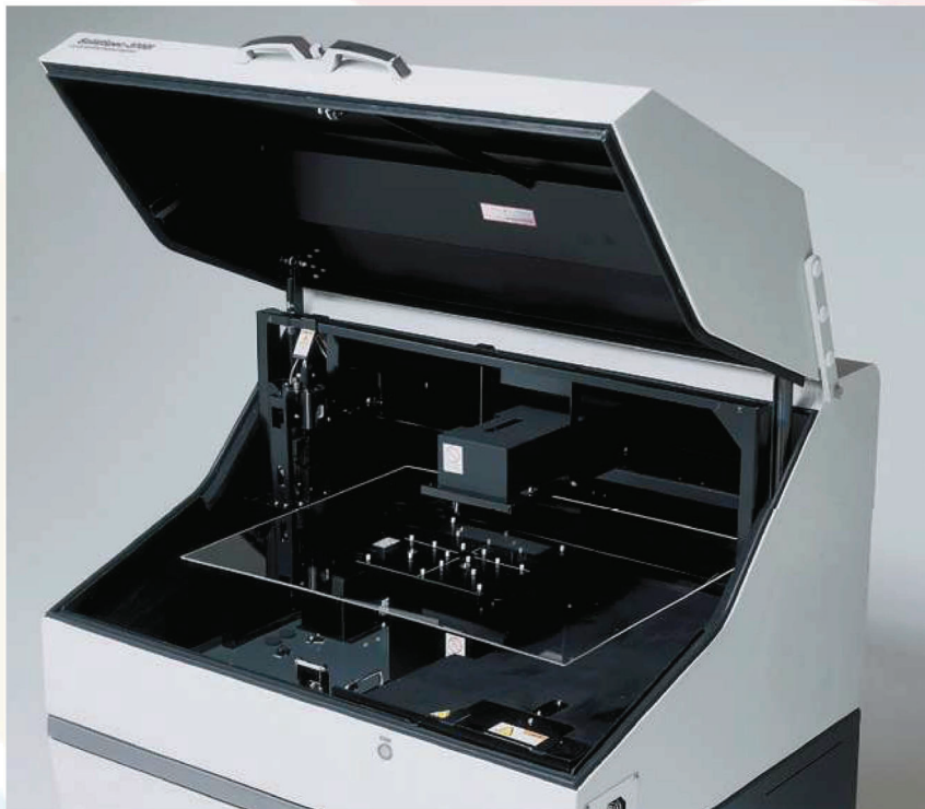
Large Sample Compartment A sample of 700W x 560D mm is set in the sample compartment.
