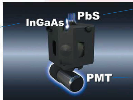
Three detectors attached to the integrating sphere
