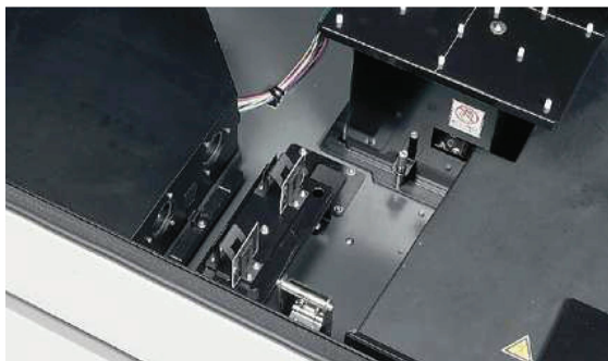
Measurement of Film Sample with Direct Detection Unit
